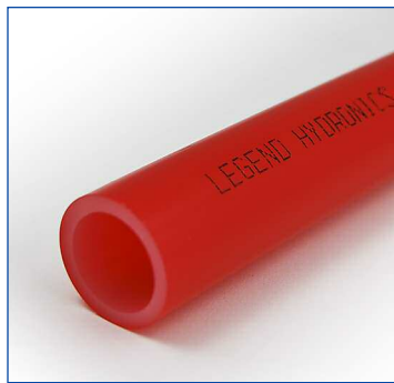
The externally-extruded EVOH oxygen barrier reduces oxygen molecule permeation into the water. Compliant with standard DIN4726 (<0.1 grams/m 3 /day)
