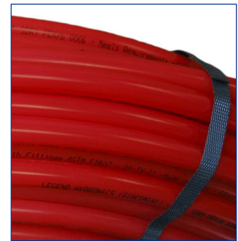
The externally-extruded EVOH oxygen barrier reduces oxygen molecule permeation into the water. Compliant with standard DIN4726 (<0.1 grams/m 3 /day)
