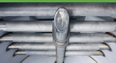
Turbo Draft System & Heat Exchange Tubes
