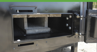
Secondary Combustion Chamber
