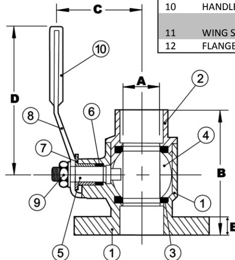
**Specifications:** Designed for residential, commercial or industrial use with water, oil or gas. This approved Webstone valve is actuated by a blowout proof stem and features an adjustable packing gland. Solder joint temperature ratings are per ASME B16.18 Annex A for 95-5 solder. Other solder materials have lower pressure/temperature limits. Do not silver braze or over heat valves when soldering.
